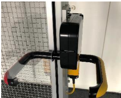
Figure 25 Escape release integrated in the handle, PSENmlock door handle module (red handle) as example
