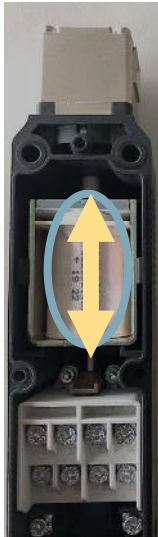
Figure 9 Interior view of electromechanical guard locking device PSEN me5
