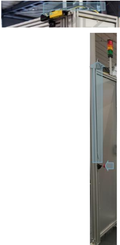
Figure 26 Escape release, using the remote escape release on the PSENmlock as an example
